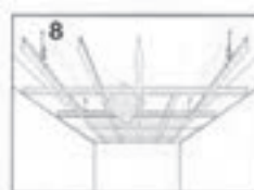
8.Installation of field and service tiles
