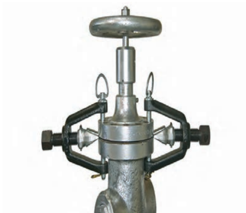
Fig 19: A flange splitter
