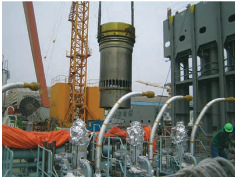
Fig 27: Big engine cylinder liner
