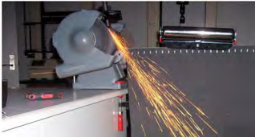
Figure 2: Spark test of a high carbon steel
