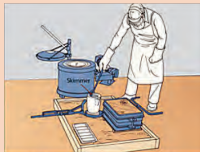
Skimming Slag from Molten Metal .....
