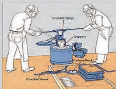
Removing a Crucible from a Furnace .....
