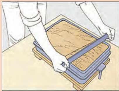
Level the Sand in the Drag .....
