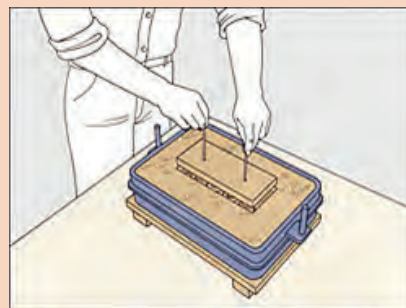
Removing the Pattern .....
