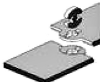
Figure 10.23. Single fillet weld
