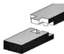
Figure 10.16. Single fillet weld
