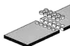
Figure 10.21. Single fillet weld
