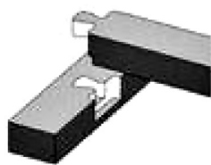
Figure 10.10. Single fillet weld
