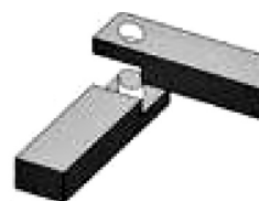
Figure 10.29. Single fillet weld
