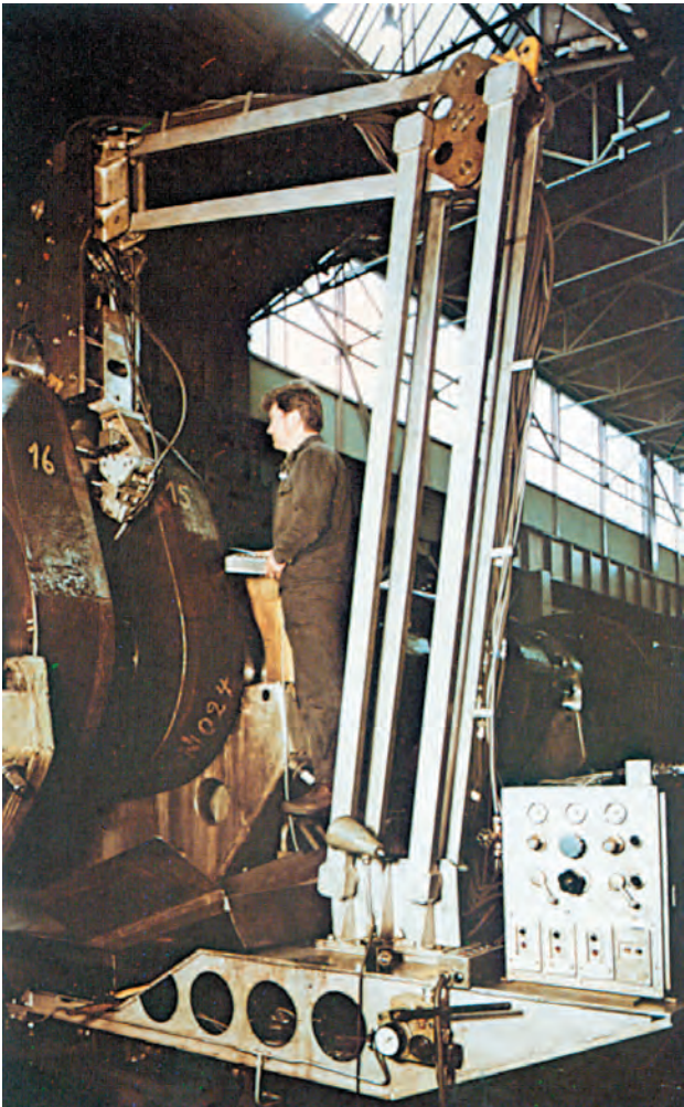
□ Machine finishing of a crank pin
